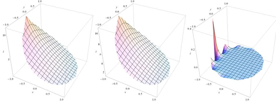
Figure 5: Example 2:  $n = 10$ : function  $u$ , interpolant  $\text{Int}(u)$ , error  $u - \text{Int}(u)$  using 21 values of Radon projections.
