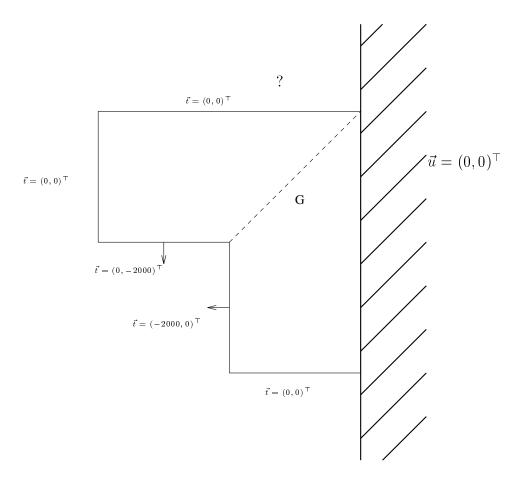
2. Partial differential equation: Linear Elasticity (plain strain)
