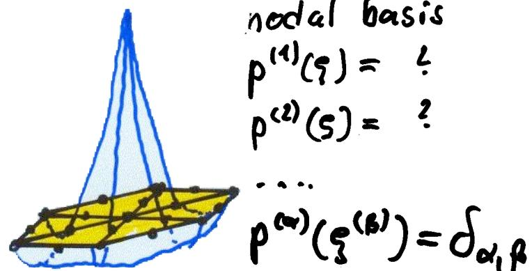
(b) cubic elements:  $\mathcal{F}(\Delta) = \mathcal{P}_3 = \text{span}\{p^{(i)}\}_{i=1,10}$
