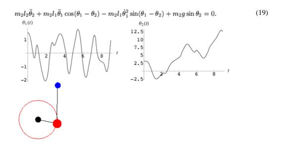
The coupled second-order ordinary differential equations (14) and (19) can be solved numerically for  $\theta_1(t)$  and  $\theta_2(t)$ , as illustrated above for one particular choice of parameters and initial
